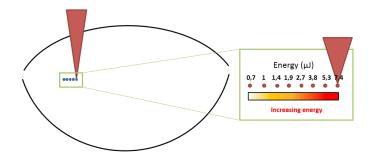
**Step 2:** Automatic detection of generated bubbles on OCT images
